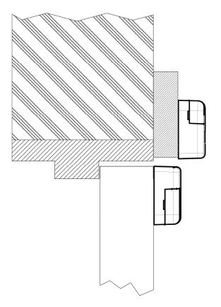
On some doors the door surround (architrave) projects forward of the door face. The IS-MDC-12 will work with the switch unit up to 8mm or more in front of the actuator unit, as shown in Figure 5. This may reduce or eliminate the need for cutting into the architrave.
