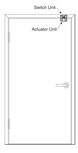
The part with the Lasermet badge and the cable attached (known as the switch) is normally affixed to the door frame, and the other part (known as the actuator) is attached to the door. The fixing hole positions are shown above and the usual mounting arrangement on a door on the left.
