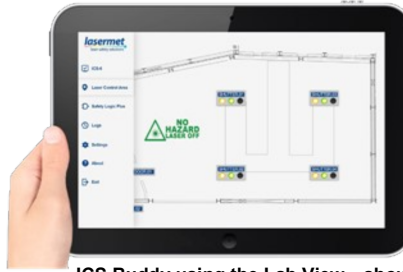
ICS Buddy using the Lab View—showing laser shutters and LED Warning sign status
